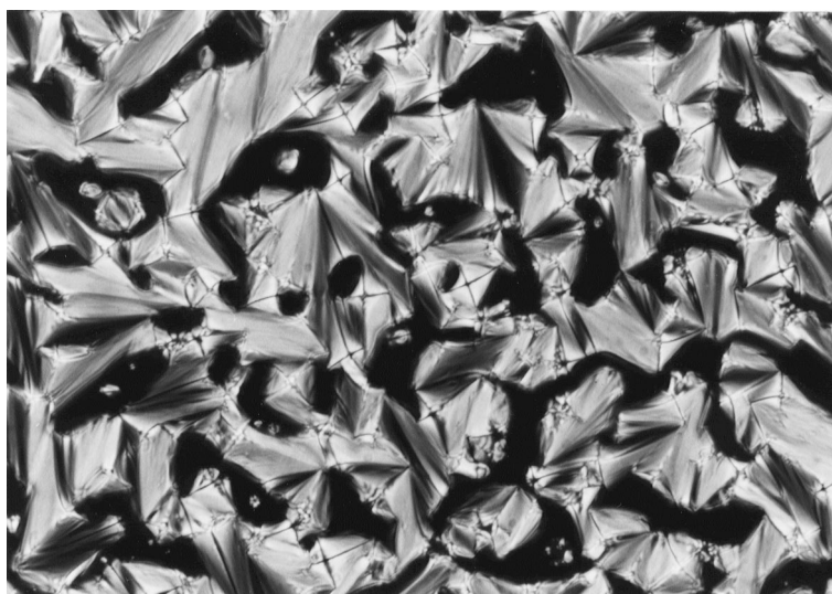
Figure 5 Smectic texture of model compound 2 2 3 (193°C, 150 ×)
